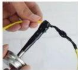
2. Apply liquid tape to wire
